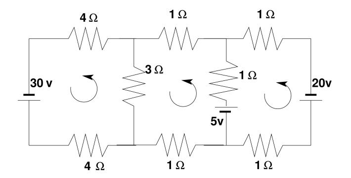
Problem: Determine the loop currents in a an electrical circuit - using Kirchhoff's Law (V = RI)
