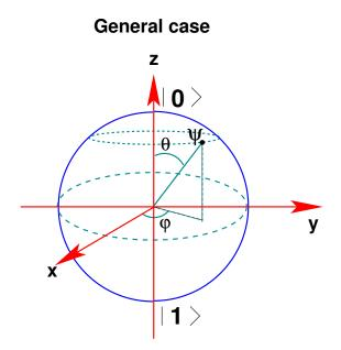
Rotation of angle  $\varphi$  around z axis.
