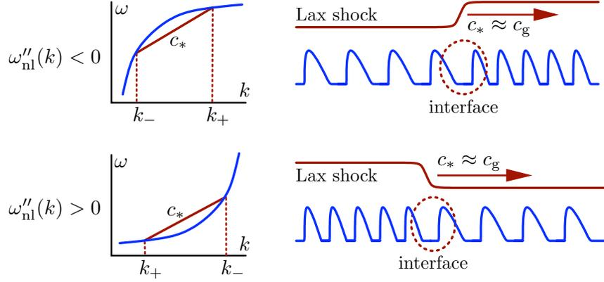
FIGURE 1.3. The relation between concave (top) and convex (bottom) dispersion relations and the resulting weak shock profiles is illustrated. The velocity  $c_*$  of the interface, given by the Rankine–Hugoniot condition (1.13) and therefore by the slopes labelled  $c_*$  in the insets, is close to the group velocity  $c_g = \omega'_{\text{nl}}$ , which is positive for the dispersion relations shown to the left.
