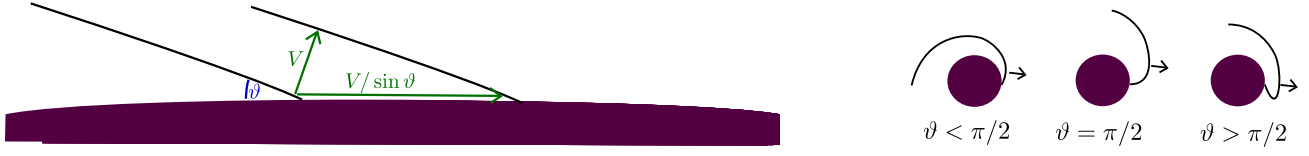
Figure 4: The limiting frequency is determined by the speed along the boundary, which is determined by the fact that its projection on the normal direction equals V (left). acute contact angles allow for monotone \Phi(r) , whereas obtuse angles induce turning points and high curvature through necessary boundary layers (right).
