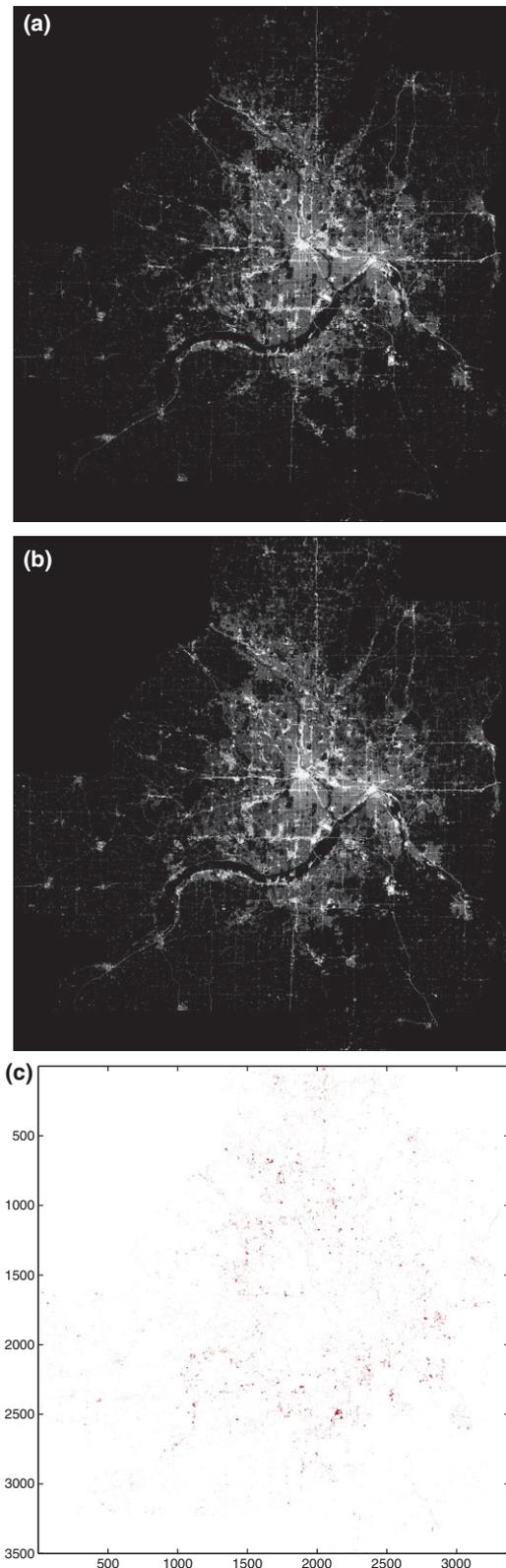
**FIGURE 11** | An example of pixel-wise change detection outputs. (a) Impervious surface image of an area in 1986. (b) Impervious surface image of the same area in 1991. (c) Locations with difference exceeding 60% of the maximum magnitude between (a) and (b).
