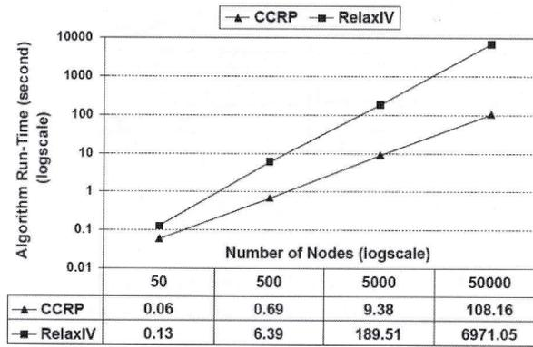
Figure 3. Run-time (log-scale) with respect to network size.
