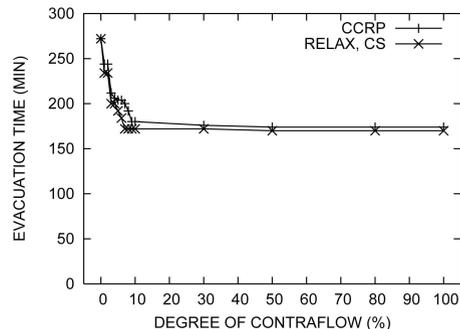
Fig. 11. Convergence pattern of the evacuation time with regard to the Degree of Contraflow using the Monticello scenario.
