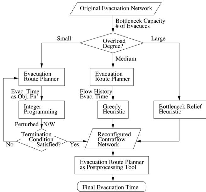
Fig. 5. Use of an evacuation route planner in the contraflow solution framework.
