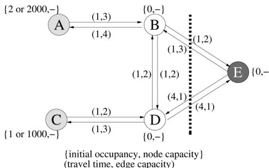
Fig. 4. Simple evacuation network with bottleneck capacity 3.
