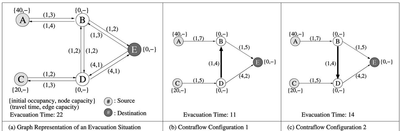
Fig. 2. Graph representation of a simple evacuation situation and two following contraflow configuration candidates. (a) Graph representation of an evacuation situation. (b) Contraflow configuration 1. (c) Contraflow configuration 2.
