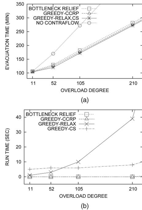
Fig. 9. Evacuation time/runtime with regard to the Overload Degree using the Monticello scenario.
