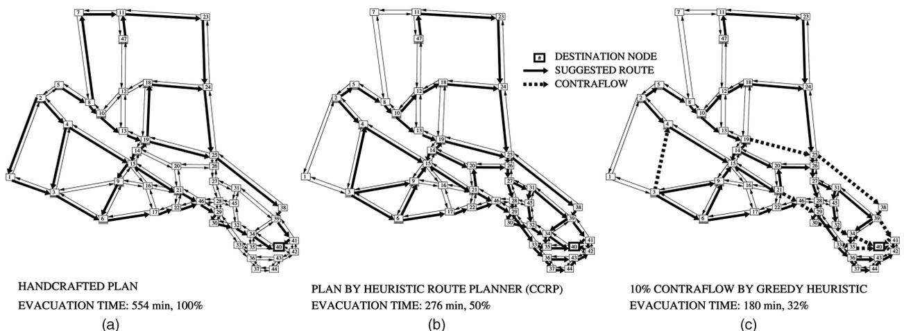
Fig. 13. Handcrafted versus computerized plans. (a) Handcrafted plan evacuation time: 554 min, 100 percent. (b) Plan by heuristic route planner (CCRP) evacuation time: 276 min, 50 percent. (c) 10 percent contraflow by greedy heuristic evacuation time: 180 min, 32 percent.
