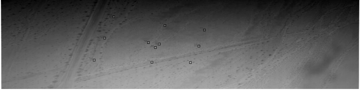
Figure 9: A sample image recorded by the camera, with the detected targets denoted by black squares.
