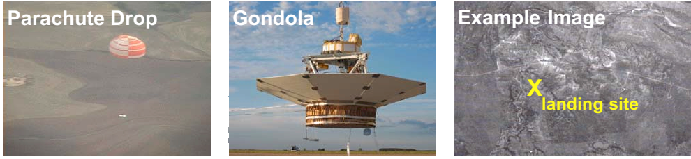
Figure 3: Pin-Point Landing Experiment on the NASA MSL Subsonic Parachute Drop Test (PDT). The gondola (center) was attached to a balloon that carried it to approximately 36 km altitude and then released it for descent on a parachute (left). During the descent, a nadir-pointing camera recorded images of the landing site (right), and an IMU provided measurements of acceleration and rotational velocity.
