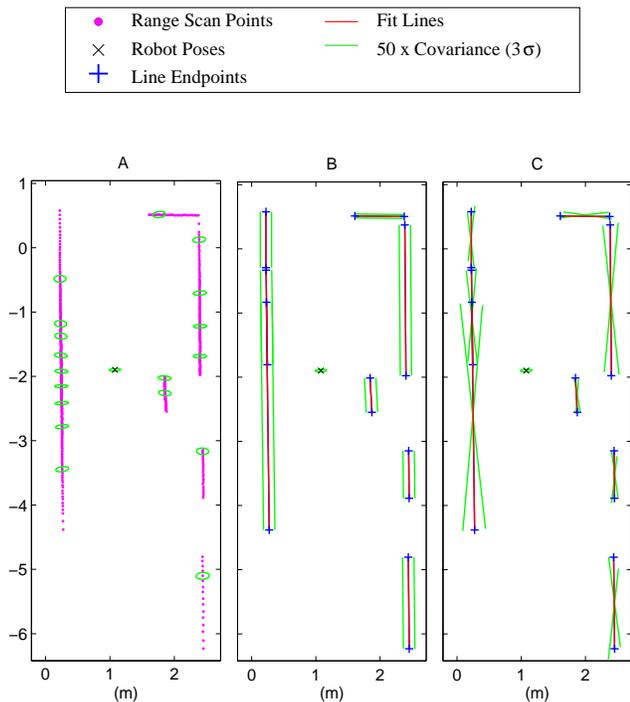
Figure 3: Range Data – A: Raw points and selected point covariances B: Fit lines and line uncertainties in R direction C: Fit lines and line uncertainties in  $\alpha$  direction
