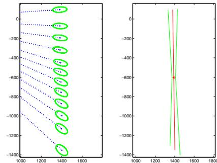
Figure 1: Example of line segment fit: data points (left) and fitted line with a representation of its uncertainty (right).
