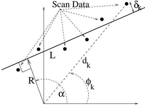
Figure 2: Geometry of candidate line and data errors
