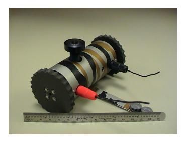
Fig. 1. A Scout robot with an upward-facing Omnitech 190° fisheye lens. The lens provides  $360^{\circ}$  horizontal field of view around the robot, effectively functioning as an omnicamera. The robot is 11 cm long and 4 cm in diameter.
