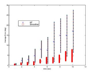
Figure 5: The average orientation error when absolute orientation measurements are available to the robot every 1, 2, ..., 10 seconds, for the case of Kalman filter (×) and smoother ( $\sigma$ ). The vertical bars represent the  $3\sigma$  intervals of statistical confidence.
