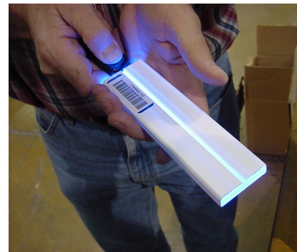
Blue LED lights up scintillator
