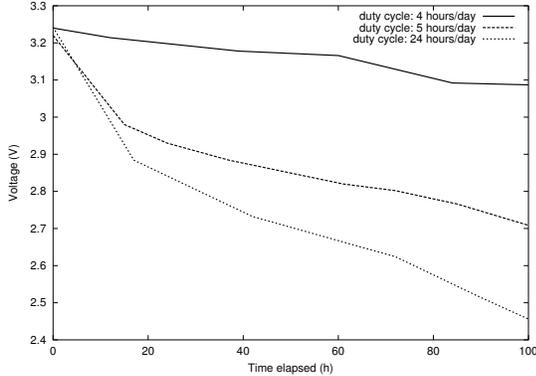
**Figure 12: Impact of Sleep Duration on Power Consumption**
