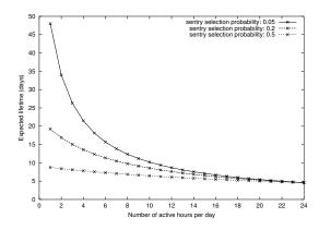
Figure 11: Expected Lifetime of a Sensor Network Using Sentry-based Power Management
