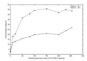
Figure 6: Impact of Sending Power on RF Range
