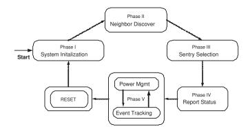
Figure 3: Time Driven System Transition
