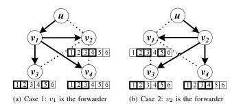
Fig. 1. Impact of coding opportunity on broadcast.In the packet reception bitmap, a block with a thick borderline means received packets, and a block with a thin borderline means a lost one.
