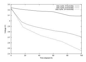
Fig. 17. Impact of Sleep Duration on Power Consumption
