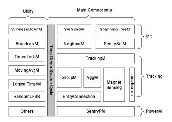
Fig. 7. System Architecture in nesC
