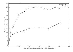
Fig. 8. Impact of Sending Power on RF Range
