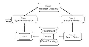
Fig. 3. Time Driven System Transition
