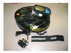
Fig. 4. GPS Mote Assembly
