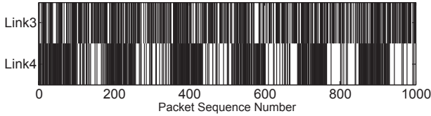
Figure 5: Temporal Correlation in real trace forces two links with similar reception ratios to exhibit different demands of 2.05 and 2.98 transmissions.
